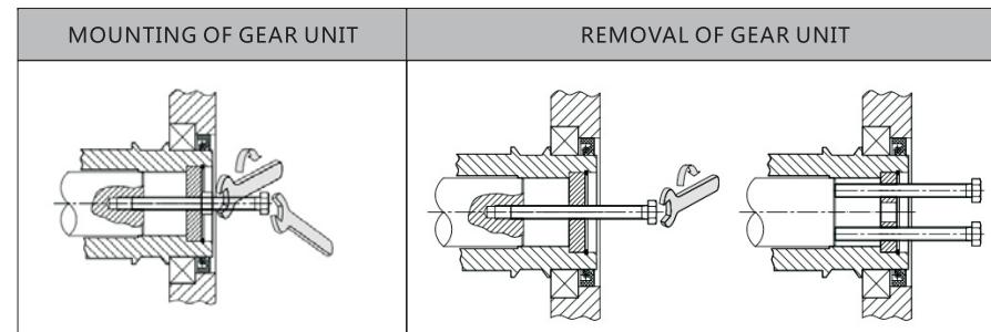
Before assembling, the contact surfaces must be clean and treated with adequate protective against rust and blocking.
